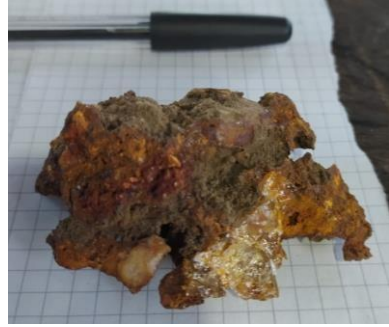
Intensely weathered pegmatites with mineralization of coltan, tin, topaz, tungsten
