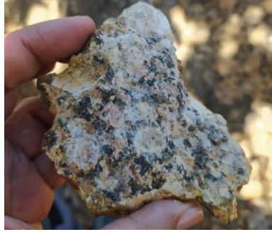
Intensely weathered pegmatites with mineralization of coltan, tin, topaz, tungsten
