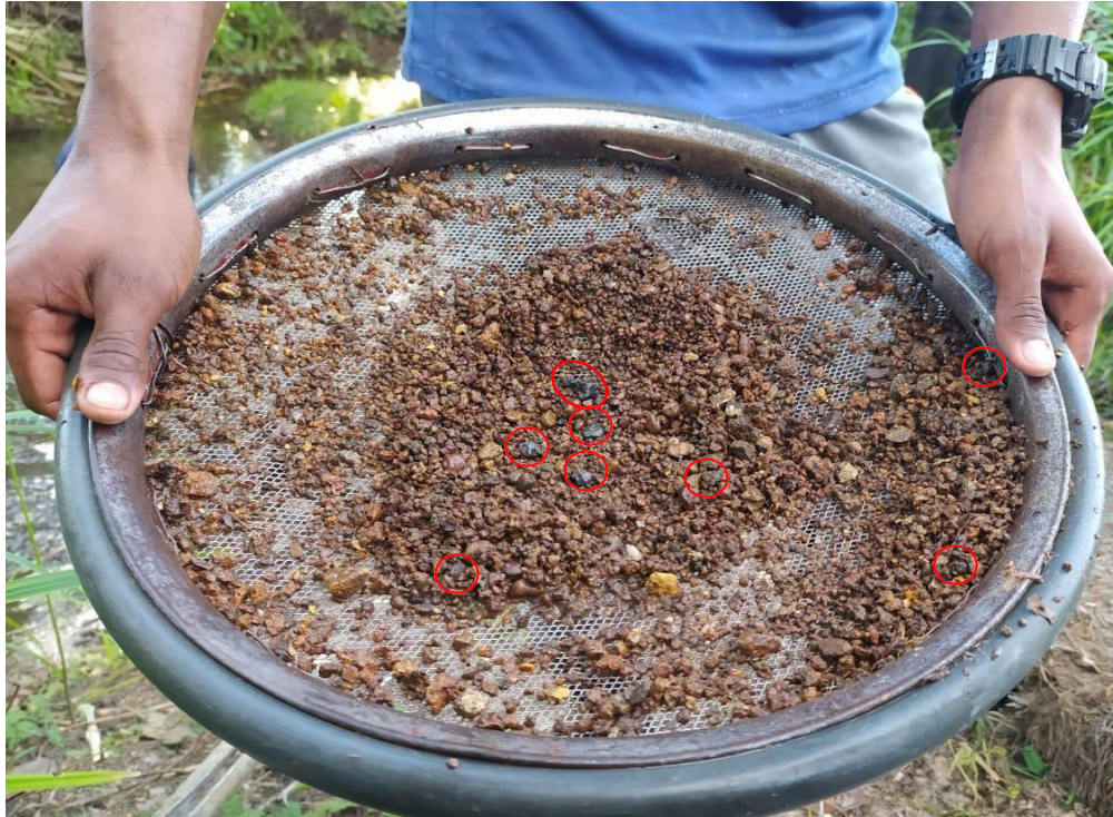
Selection of the material by batting in the area of interest of Venezuela. Coltan fragments circled in red
