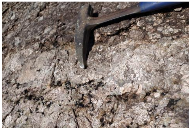
Quartz veins with micas, coltan and tin mineralization.
