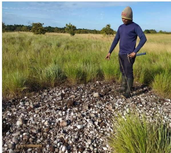
Eluvial and alluvial placer deposits. This is the type of deposit of greatest interest to the locals as the exploitation requirements are minimal. Observe the amount of quartz fragments in the ore veins.
