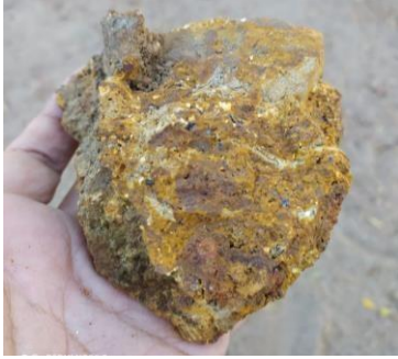
Intensely weathered pegmatites with mineralization of coltan, tin, topaz, tungsten
