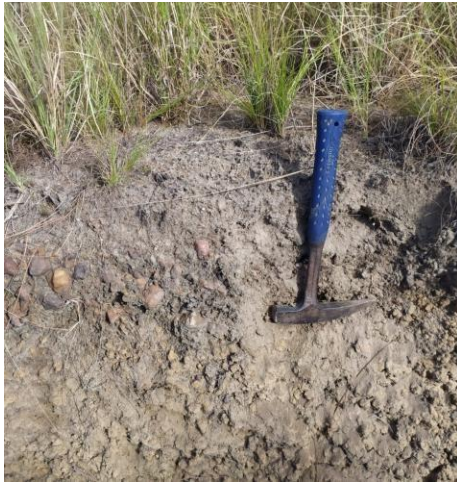
Intensely weathered pegmatites with mineralization of coltan, tin, topaz, tungsten
