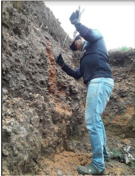
Photo 5 & 6. Photo and detail of the tricheras in the alluvial plain where coltan and tin material has been extracted. Channels were made to take the samples, even so the best results were presented on selected fragments.
