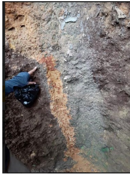
Photo 5 & 6. Photo and detail of the tricheras in the alluvial plain where coltan and tin material has been extracted. Channels were made to take the samples, even so the best results were presented on selected fragments.
