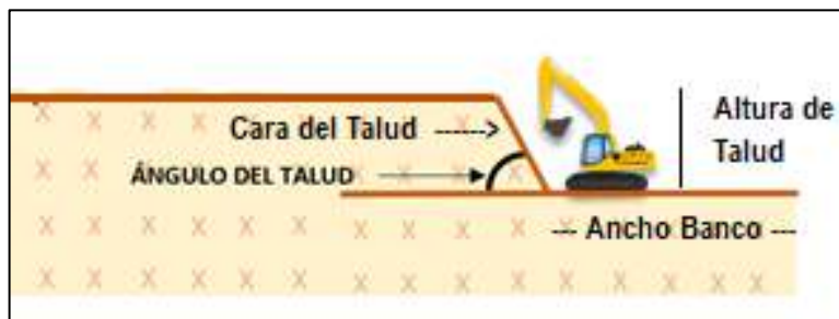
Figure 15. Geometry of an open pit mine
